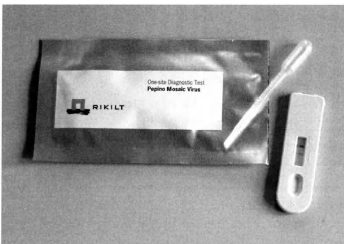
Figure 8 For storage, the strip test is packed into a foil pouch in the presence of a sachet with some kind of dessicant, e. g., 1 g silica gel MiniPax. In this way, the strip tests can be stored for several months at ambient temperature without serious loss of quality. When the assay will be used to test liquid samples, a small pipet may be included as well.
