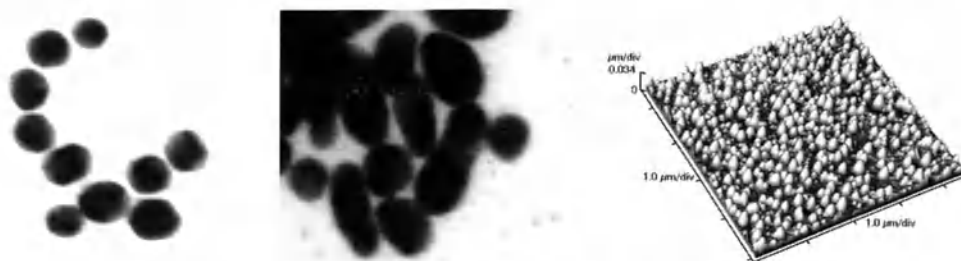
Figure 1 Nano-cluster: crystalline and amorphous via chemical synthesis (left, middle) and sputter coated (right)
