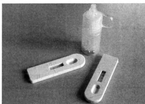
Figure 9 When the assay will be used to test solid samples (plant leaves, solid food, or feed samples, etc.), a simple extraction procedure has to be included. This can be achieved by placing a certain amount of sample material into a small bottle with dropper cap that contains a few milliliters of extraction buffer and five or six stainless steel ball bearings. After having shaken the bottle firmly for 20 to 30 s, a few drops of extract are brought into the sample well.
